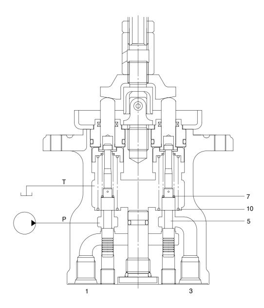
The force of the spring(7) that determines the output pressure of the pilot valve is not applied to the spool(5). Therefore, the spool is pushed up by the spring(10) to the position of port(1, 3) in the operation explanation drawing. Then, since the output port is connected to tank port T only, the output port pressure becomes equal to tank pressure.
